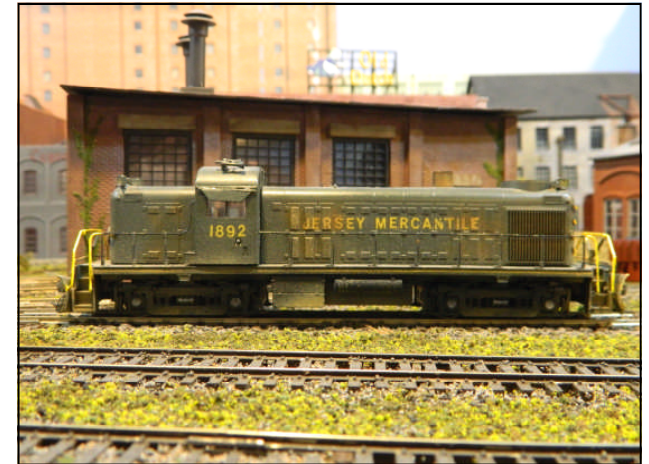
Locomotive 1892 is an ALCO RS2 which has the fuel filler cap on the side of the cab (seen under the 92 numbers. This is a Kato model.
