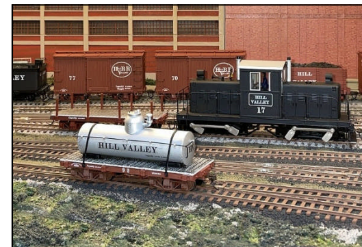
The only active diesel on the Hill Valley is seen in Wallington yard performing switching duties for the next outbound local. It is a 50-ton Whitcomb centre cab unit employing side rods on its driving wheels (Bachmann On30).
