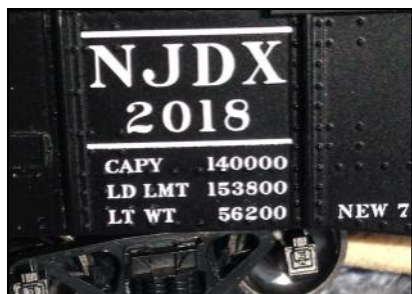
The Reporting Marks "NJDX" for this car identify the owner as the New Jersey Division and the "X" designates a Private or Non-railroad owner.
