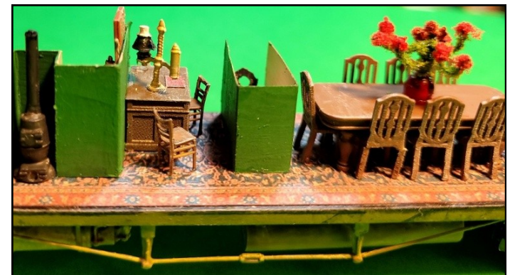
View of office area and truss rod on underframe
